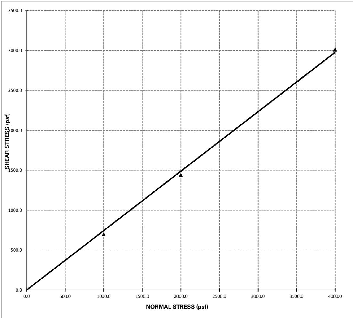
**Shear Strength:**  $\Phi = 36.6^\circ$  ; **C = 0.00 psf**
