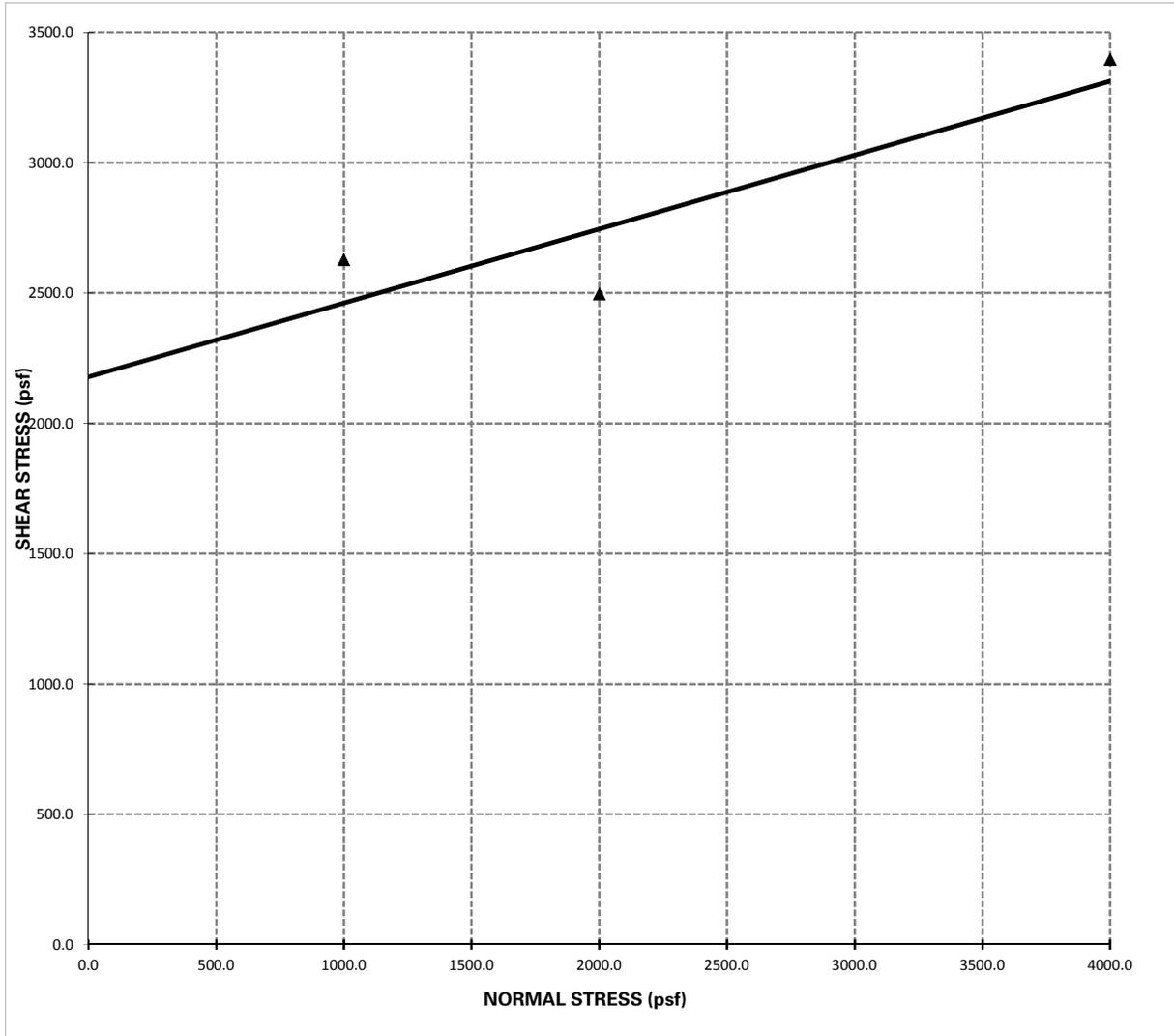
**Shear Strength:**  $\Phi = 15.8^\circ$  ; **C = 2178.0 psf**
